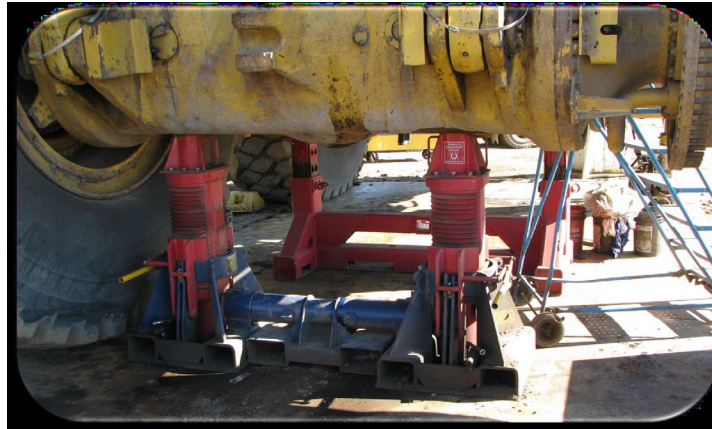
TriLift Jack Stand positioned under haul truck axle housing
