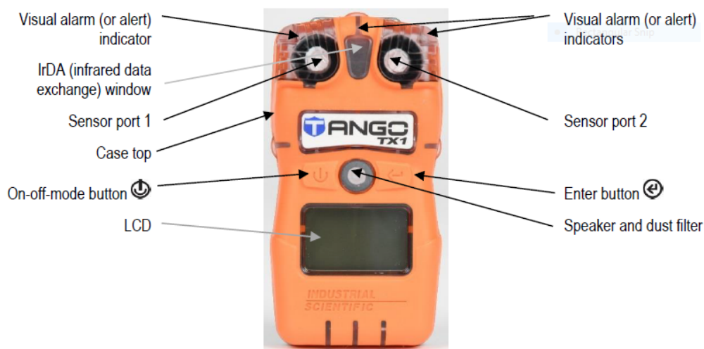
Figure 6-2 Tango TX1 Single Gas Monitor Overview
